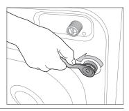
2. Hold the bolt with the spanner and pull it through the wide section of the hole. Repeat for each bolt.
