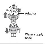
2. First, using a '+' type screwdriver, loosen the four screws on the adaptor. Next, take the adaptor and turn part (2) following the arrow until there is a 5 mm gap.
