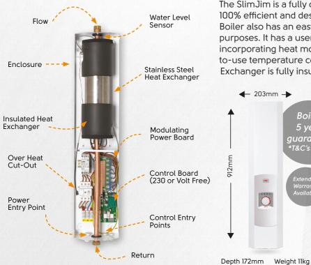
The SlimJim is a fully controllable Electric Flow Boiler which is 100% efficient and designed to maximise cupboard space. The Boiler also has an easy-fit front cover for future maintenance purposes. It has a user-friendly Front Control Panel incorporating heat mode and fault finding indicators and easyto-use temperature control setting. The stainless steel Heat Exchanger is fully insulated to minimise heatloss.
