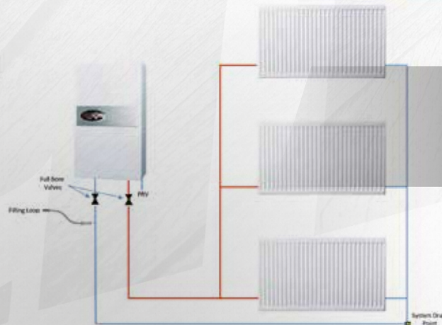
Heating only with Direct Cylinder Hot Water design
